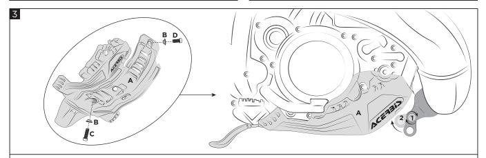
Place the Acerbis skid plate (A) on the frame and secure it using two bushings (B), the screw (C) and the screw (D). Then re-insert the screw (2) and tighten the screw (1).
